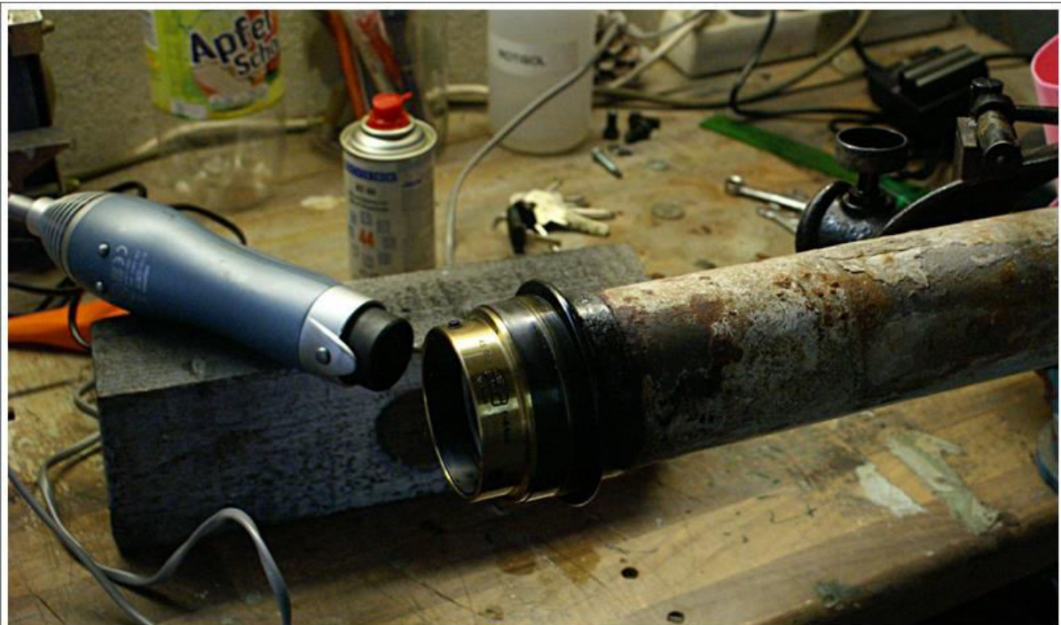
Zeiss Asegur dewcap uninstalled after 4 days influence of WD-40 and working with hair-dryer !
